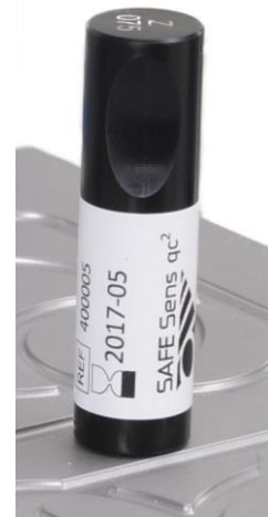
SAFE Sens® qc 2 alignment tool on TrakPod™'s sv 2 -sensor in benchtop incubator Labo C-Top
